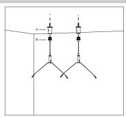
③ Hanging the panel light to the suspending wires, connect the DC plug between driver and panel light.
